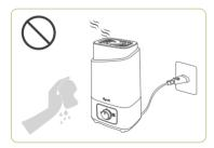
DO NOT clean the humidifier immediately after turning it off. Allow the humidifier to cool down completely before cleaning.
